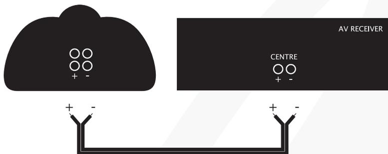
The binding posts on the terminal accepts wire up to Ø 4mm. Make sure that the positive terminal binding posts on CinePod (+) are connected to the positive output terminal binding posts on the amplifier and that the negative terminals on CinePod (-) are connected to the negative output terminal on the amplifier.
